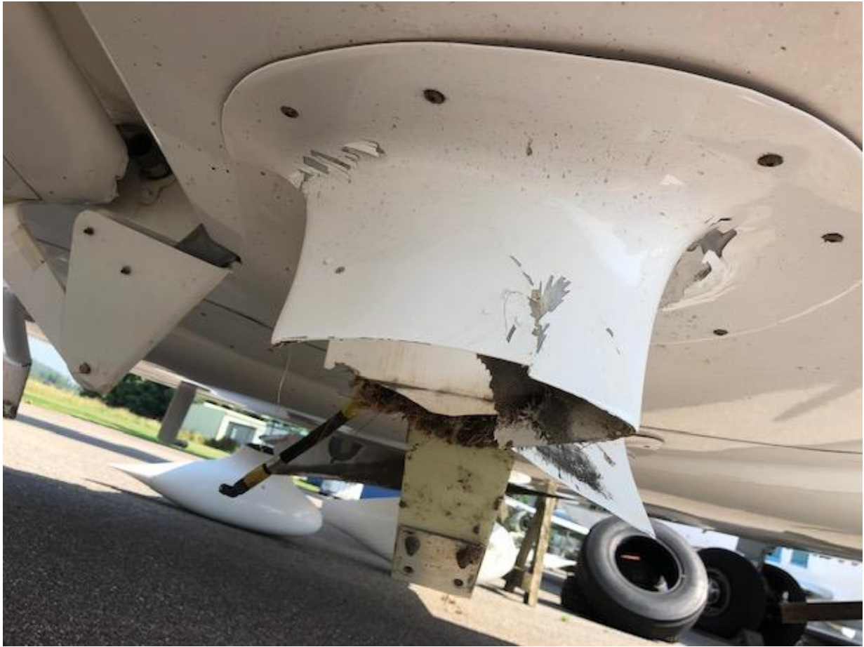
Right main landing gear wheel has detached
