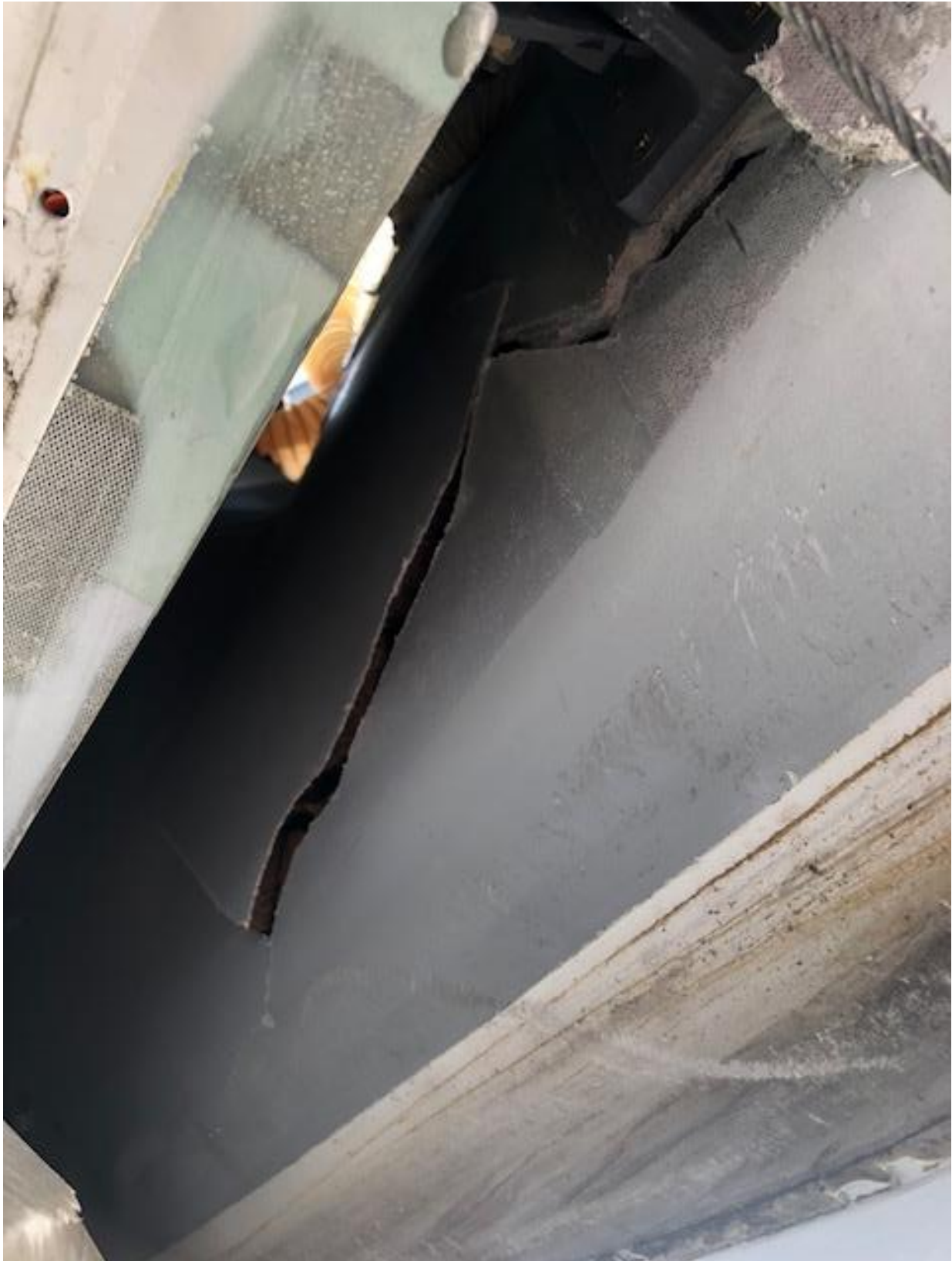
View of left fuselage where left wing attaches showing extensive damage
