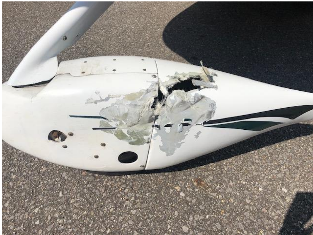
Damage to nose leg
