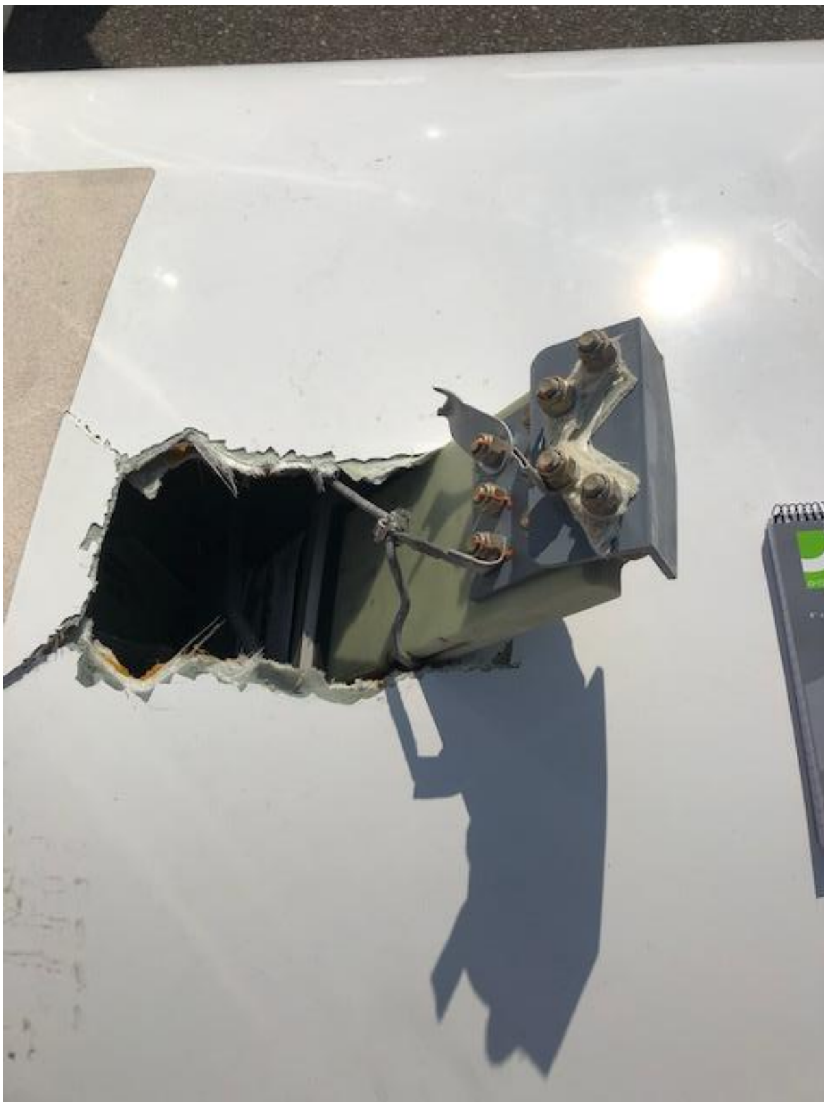
Right main landing gear has punctured through top skin of wing (aft looking forwards)
