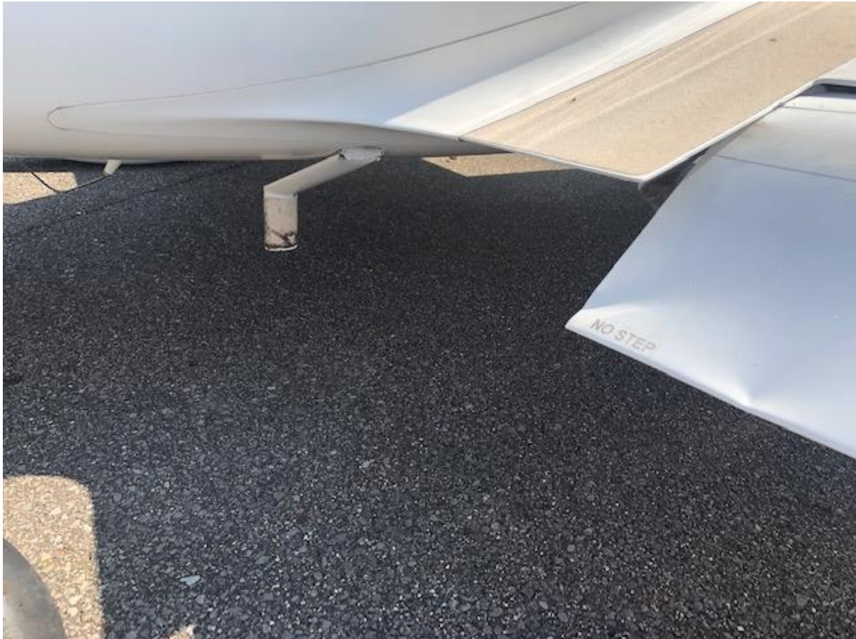
Right access step damage
