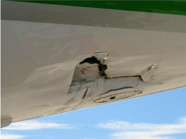
***Puncture and tear to fuselage skin at station 743***
