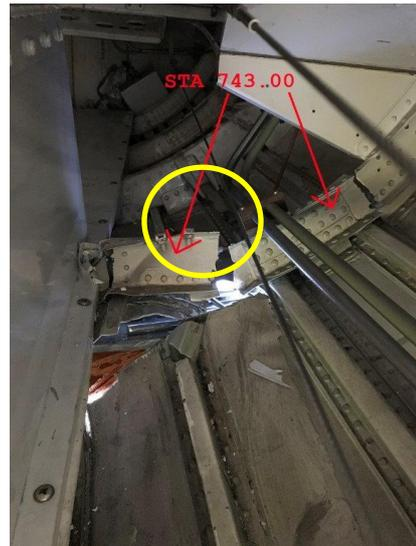
***The frame at station 743 has cracked***
